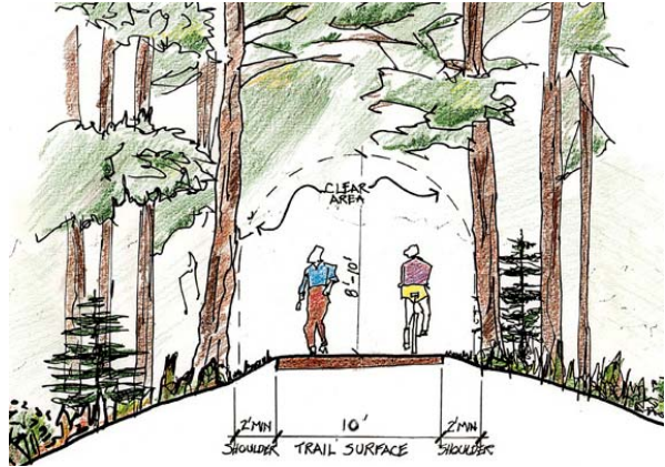
Image 11 – Typical design standards for main trail system – SAA 2010
