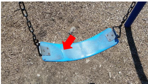
Belt swing seats are damaged
