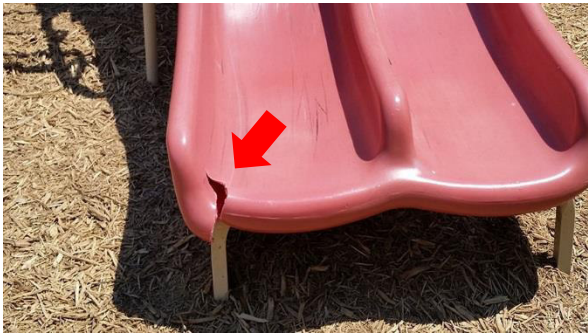
Cracked play structure slide
