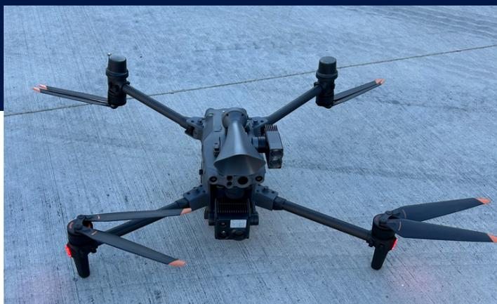
All the drones are fully equipped with a thermal, wide-angle, and high resolution optical camera. They also have the ability to record video. A laser rangefinder and speaker/spotlight are installed on each drone as well.
