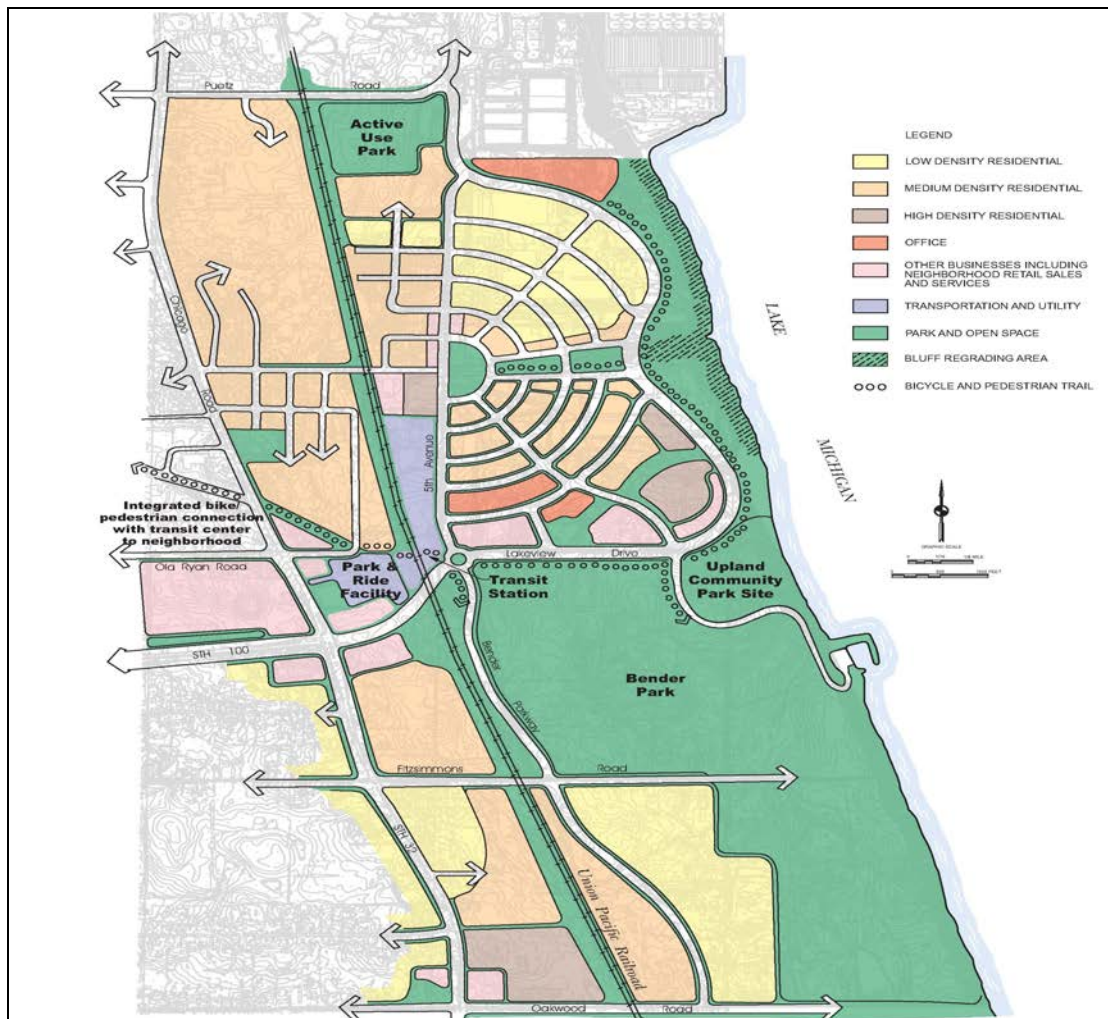
FIGURE 11-1 EXAMPLE OF A NEIGHBORHOOD DEVELOPMENT PLAN INCORPORATING TRANSIT-ORIENTED DESIGN PRINCIPLES
